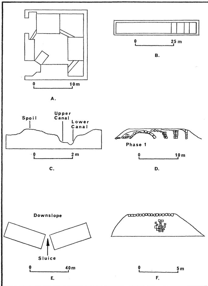
Figure 3 Schematic diagrams of water control features: (a) Cañada Norte settling tank; (b) Atzompa settling tank; (c) Main Xoxocotlan canal; (d) Cañada Norte dam; (e) Xoxocotlandam; (f) Xoxocotlan dam
